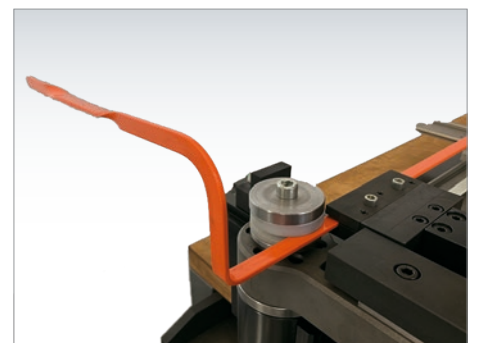
Bending / twisting copper
