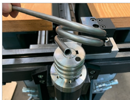
Tight spiral (spiral bending)
