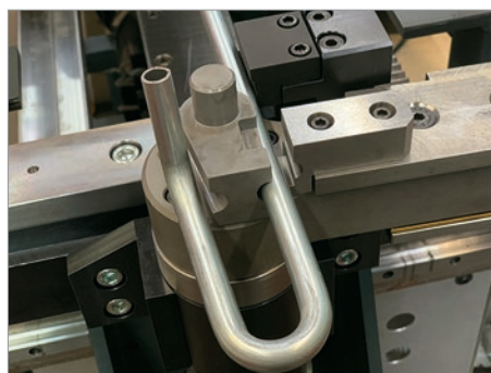
Bending with booster 1.2 x D
