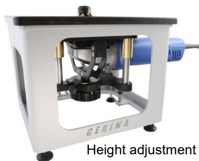
Milling head with 3 carbide inserts for bevel and guiding roll
