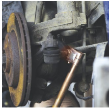
Loosening track rods
